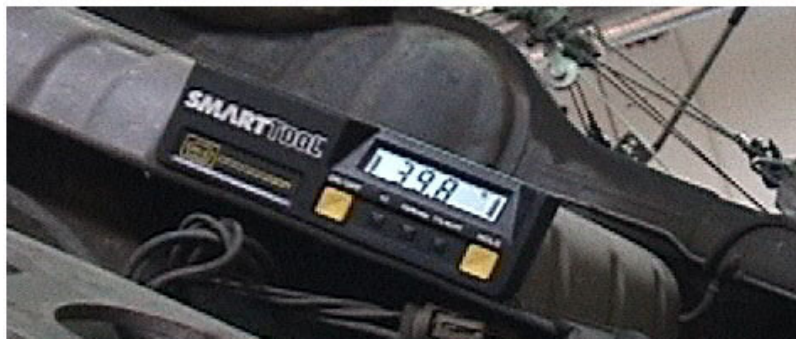
FIGURE 7. PRE-TEST ROLL ANGLE MEASUREMENT
